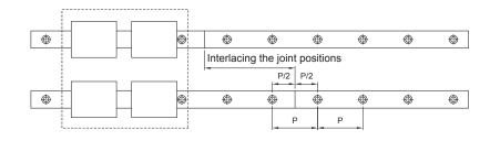
Fig.9 Staggering the joint position
