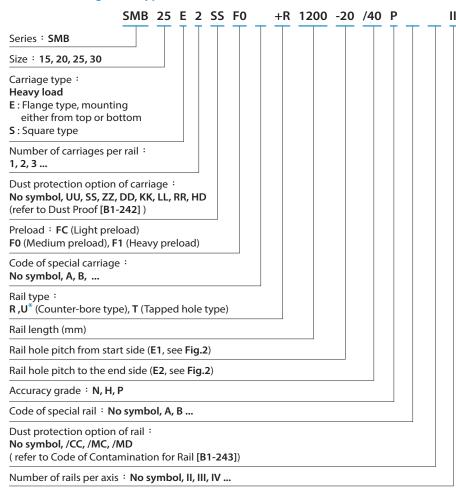
Note\*: U type rail is only applicable for MSB15 with M4 mounting hole.
