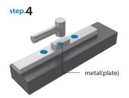
Continue pounding the cap until the cap is on the same plane with the top surface of rail.
