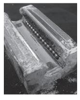
After running 150 KM in a wood flour test environment, the carriage is still moving smoothly and the steel balls are also glossy. The end seal and inner seal protect against wood flour from entering the carriage. Overall running smoothness is not effected.
