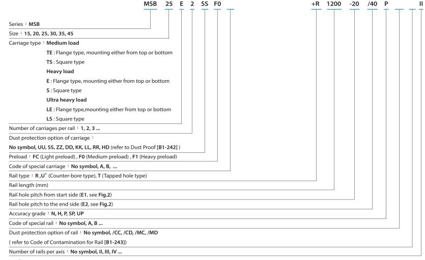
Note\*: U type rail is only applicable for MSB15 with M4 mounting hole.
