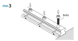
Check for correct bolt play and temporarily tighten all bolts.
