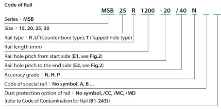
Note\*: U type rail is only applicable for MSB15 with M4 mounting hole.
