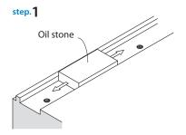
Prior to installation, the burrs, dirt, and rust preventive oil should be removed thoroughly.
