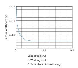
Relationship between working load and friction coefficient
