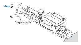
Tighten all bolts to the specified torque. The tightening sequence should start from the right side to the left side. By doing this, the original accuracy could be achieved.
