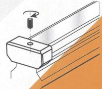
Position the protective cap at the end of rail and tighten the setscrew.
