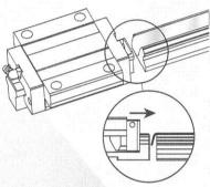
Position the carriage, with its jig inserted, at one end of the rail. Push the carriage onto the rail and the jig will be pushed out of the carriage by the rail.
