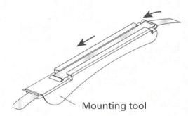
By the arrow direction, put the band through the mounting tool.
