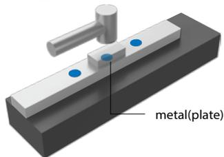
Put the plate on the cap, then pound it into the bolt of rail with rubber hammer vertically.
