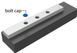
Put the cap into the bolt hole of rail.
