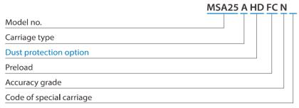
Note: Rail Model- MSA15, MSA20, MSA25, MSA30, MSA35, MSB15, MSB20(A type, E type, S type)
